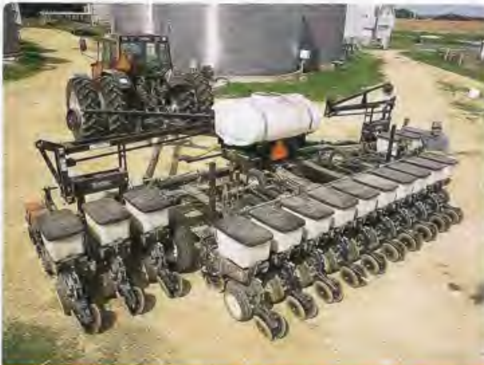
A 16-row, 20" planter built by farmer and Extension researcher Jim Leverich no-tills through heavy residue and never plants in a wheel track.
