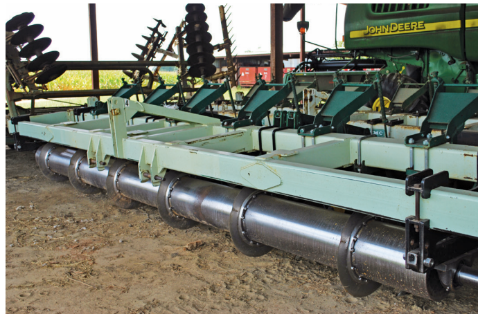
SHOP-MADE STRIP-TILL RIG. Myron Johnson invented a strip-till rig with a roller to terminate covers while making strips for cash crops. Blades mounted on the pipe roll down and cut the cover crop in front of shanks that create strips. Rubber closing wheels seal up the seed trench, followed by a set of five rubber tires that are 12 inches tall and 10 inches wide that smooth the soil out.
