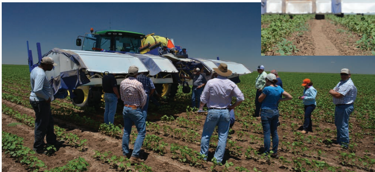
SPOT ON. Blue River Technology and John Deere have developed "see and spray" technology that identifies individual plants to determine whether they are weeds or the crop, and then takes action based on that information, says Alex Purdy, the head of John Deere Labs, based in San Francisco.
