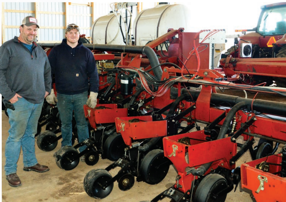
OPTIMIZING SEEDING. Jeff Lake (left) and his son, Jake, no-till 1,500 acres of sandy soils in northwestern Wisconsin. The Lakes use EFC Systems’ Profit Zone Manager tool to help them optimize variable-rate corn seeding rates between 18,000 and 32,000 with their 16-row Case IH 1200 Early Riser planter.
