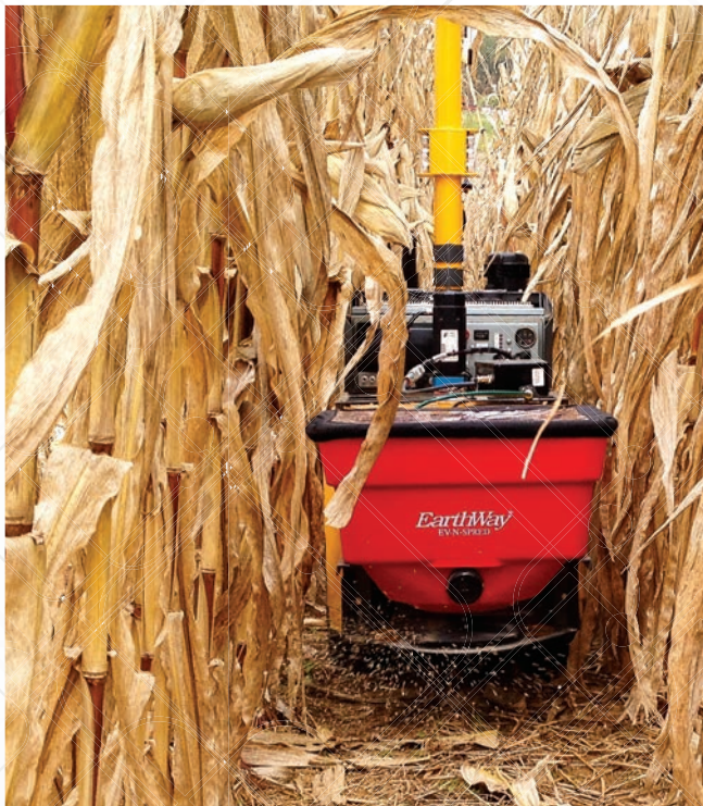
ROW RUNNERS. No-tillers may interseed cover crops a few weeks ahead of harvesting corn or soybeans with units that run between the rows under the growing crop.
