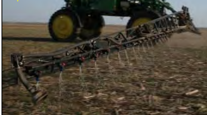
3 hole fertilizer caps can streak a field, especially when operated at higher forward speeds. These nozzles were operated around the recommended height above the crop and still streaked the field.
