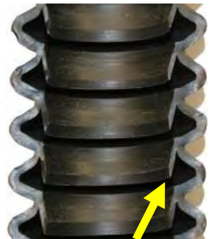
Cross-section of a stretched seed tube, showing the folds.
