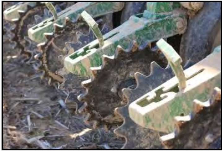
The Needham Ag Poly 20 Point Wheels being used on a John Deere DB 60. This field was corn after corn and the field had been vertical tilled. Minimal down pressure was needed to close the seed slot within these conditions.
