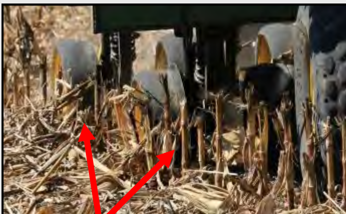
The Problem: Wide gauge wheels are lifted by corn stalks, resulting in shallow seeding depth and potential winterkill in crops like winter wheat.
