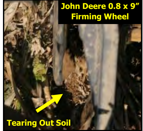
John Deere 0.8 x 9" Firming Wheel Tire Coming Off The Rims. Our V8 Tire Can't Come Off, As The Bolts Go Through The Tire.
