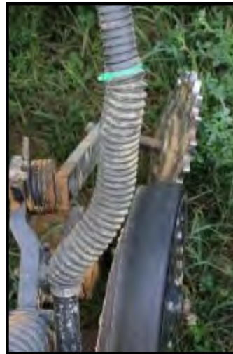
Radish seeds hanging in a factory seed tube angled at only 30 degrees from vertical.
