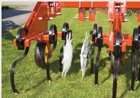
Split row shields allow safe controlled return of soil to plants. Fully adjustable.
