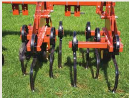
Units can be converted easily to field cultivators by adding additional tines. Shields or hillers must be removed.
