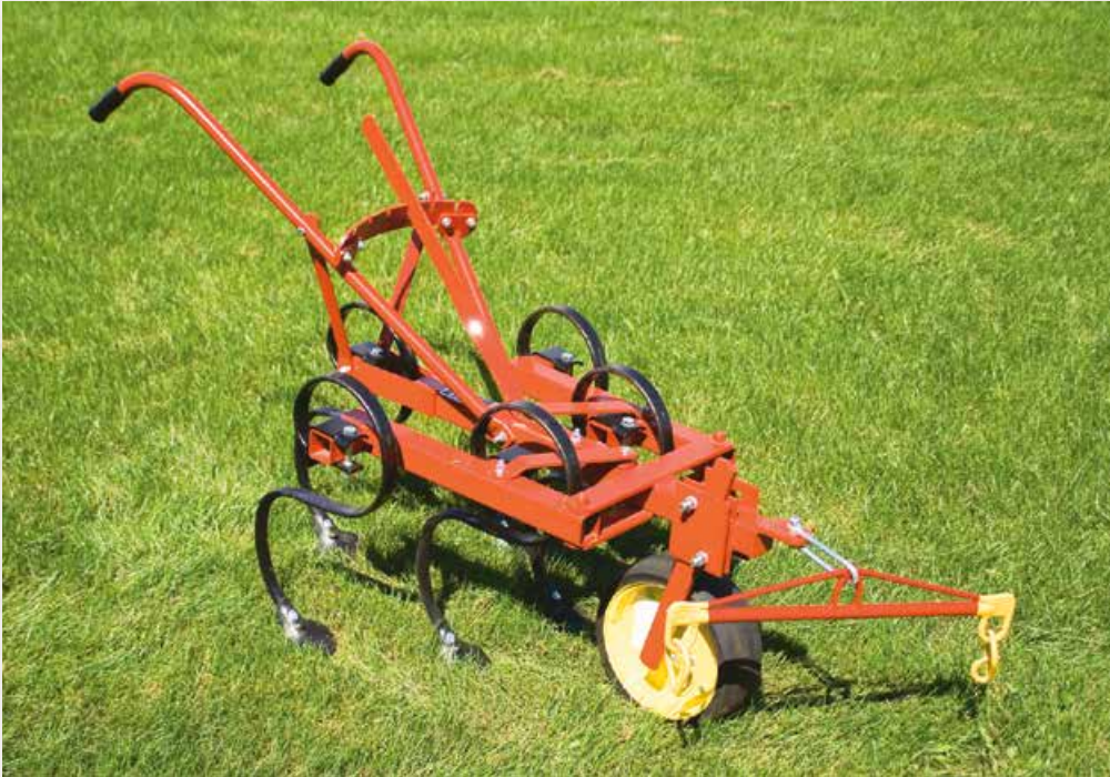
Five Tine Cultivator has adjustable row width for use with horse or pony.
