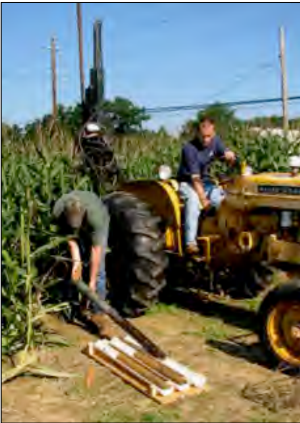
Taking soil core to a depth of 2 ft (60 cm)
